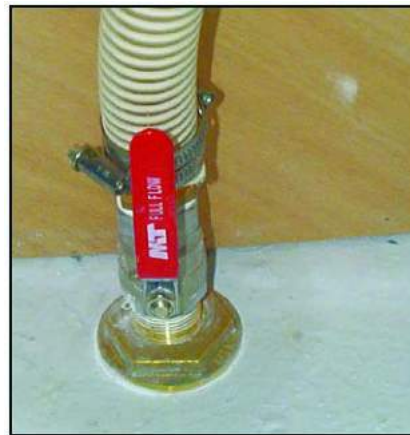
Thru-hull fitting open
