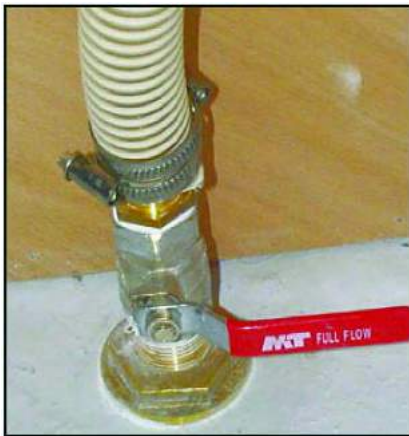
Thru-hull fitting closed
